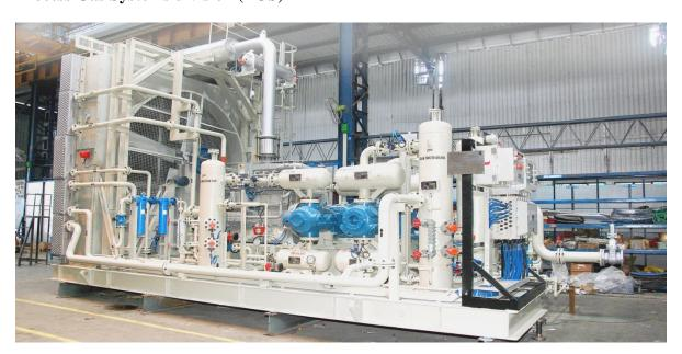
PGS provides turnkey solutions for Gas Compression Systems in the Oil and Gas Sectors. It also undertakes Operation and Maintenance contracts for Compressed Natural Gas (CNG) and American Petroleum Institute (API) Gas Compression packages. KPCL offers CNG packages with Suction Pressure (0.5 to 65 bars) and Gas Flow (300 to 3,500 SCMH). API Gas Compression packages range from 50 CFM to 6000 CFM.
